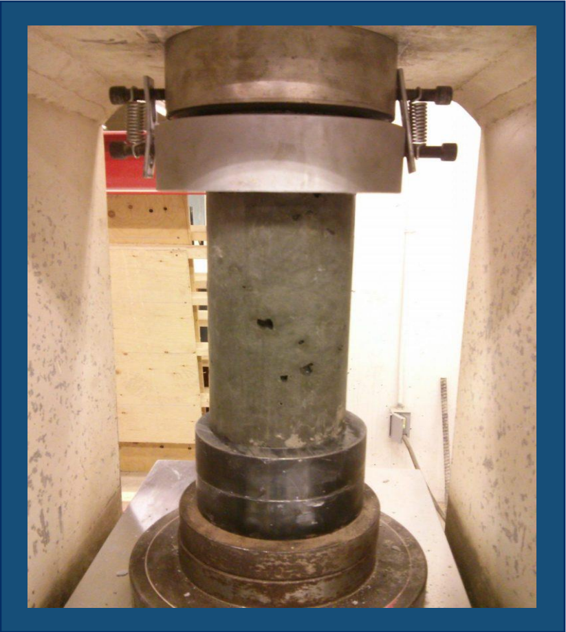
Figure 5- Example Concrete Cylinder Strength Testing [7]
